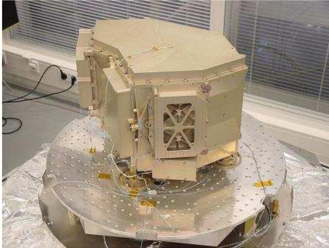
*Figure 4.* The MIRI spectrometer main optics for the JWST satellite in the NOVA Op-IR instrumentation group located at ASTRON. (Courtesy NOVA)
