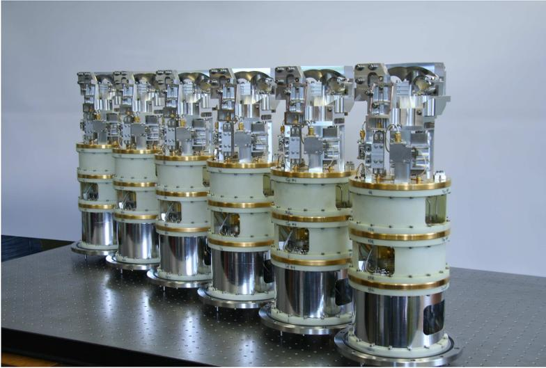
*Figure 1.* Six of the 73 ALMA Band-9 cartridges, a main part of the Dutch contribution to the ALMA project, designed and produced in a collaboration between NOVA, SRON and TuD. (Courtesy NOVA)
